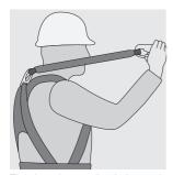
The dorsal extension is located at the rear of the harness, held in place by velcro strip
