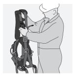
Hold harness by the shoulder straps and disconnect the chest fast release buckle
