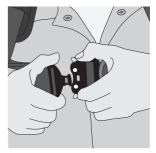
To release, push the two side tabs simultaneously and separate the buckles
