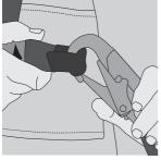
Connect attachment hardware to the eye, making a visual check for secure connection
