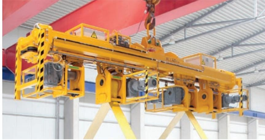
The flexible rotation beam is also suitable for heavy loads
