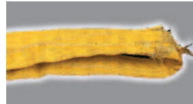
Only the sling reinforcement is damaged
