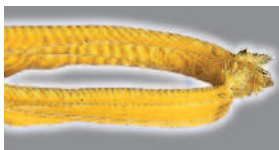
Damage to the slings (not the reinforcement)
