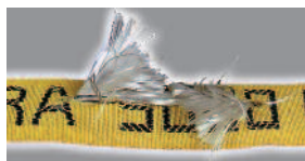
Damage to the internal strands
