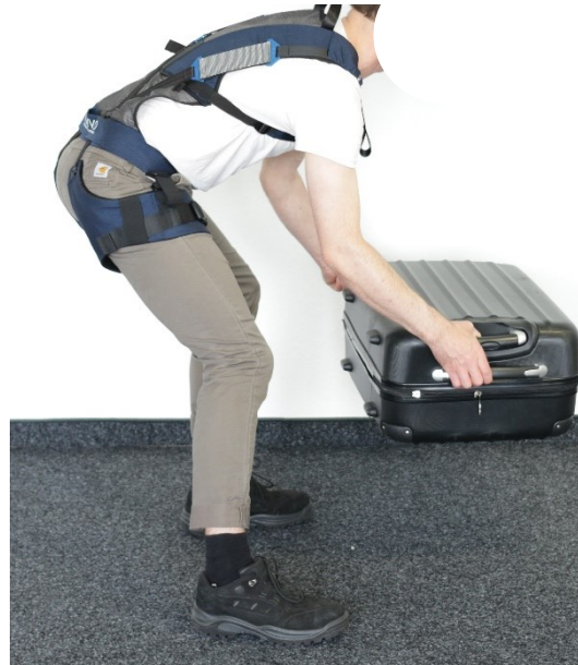
When you lean forward for a deep lift, the preload on the elastic energy storage elements can be lower. It should not restrict you from bending down.
