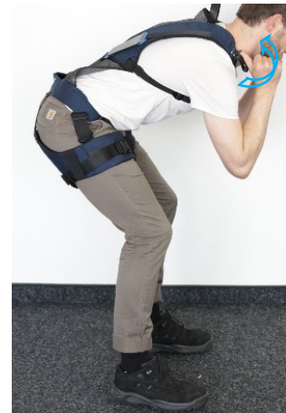
Deactivate the system by tilting the activation buckles with your thumbs, while remaining in the forward-leaning position.
