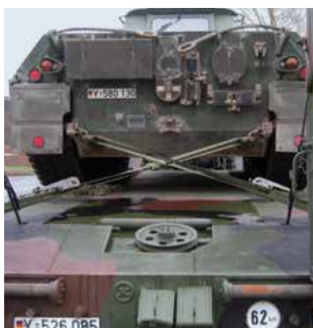
High performance direct lashings for NATO tanks
