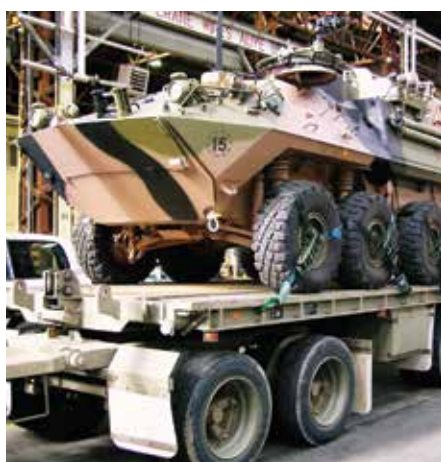
ASLAV 8WD amphibious vehicle wheel restraints
