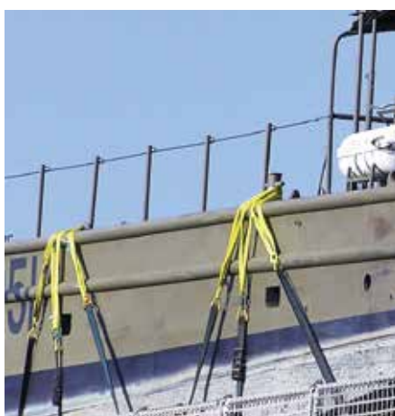
Round slings used as redirecting anchorages on HMAS Kanimbla
