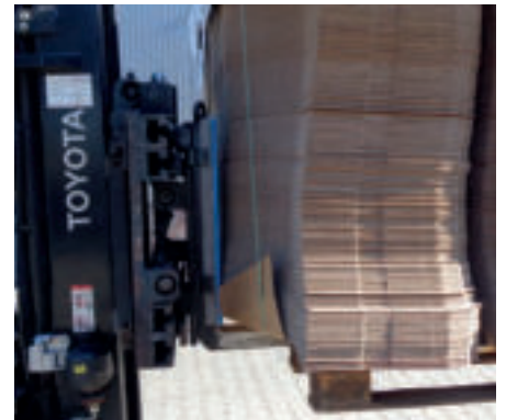
secutex soft fork rear impact cushions for transporting fragile goods such as roof tiles or plasterboard.
