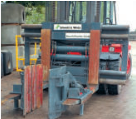
The secutex pipe gripper enables manhole pipes to be transported safely and carefully. Surface damage is reliably prevented.
