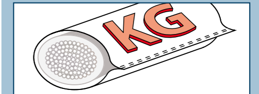
Raised, woven-in load capacity specification.
