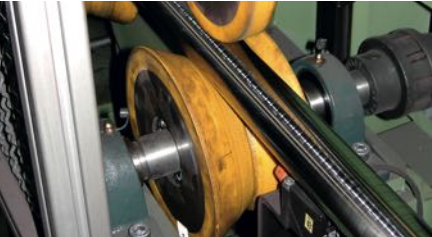
Guide and pressure rollers with exchangeable cores
