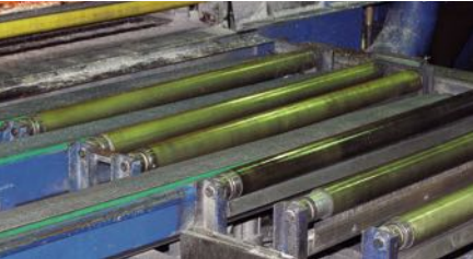
Rollers for the transport of sensitive profiles
